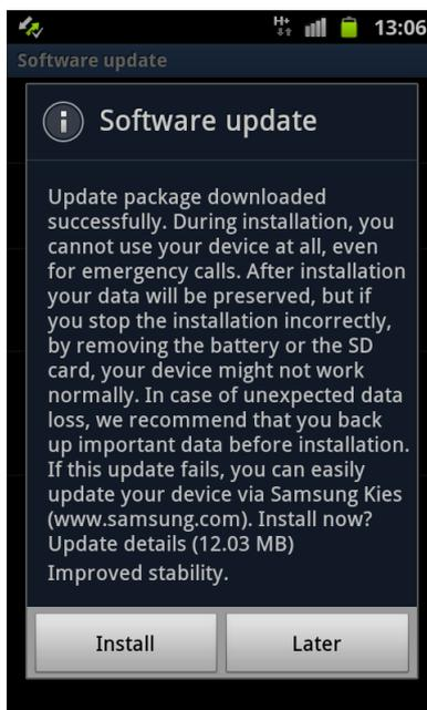
8. Select "Install". The mobile phone will now switch off, restart automatically and install the software. Please wait until the installation is complete. At the end of the installation process, the mobile phone will switch off automatically and restart one more time.
